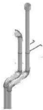
Single Pipe exhaust venting with straight pipe (C)PVC or PP termination.
